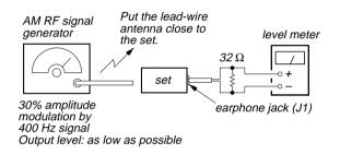
• Repeat the procedures in each adjustment several times, and the frequency coverage and tracking adjustments should be finally done by the trimmer capacitors.
