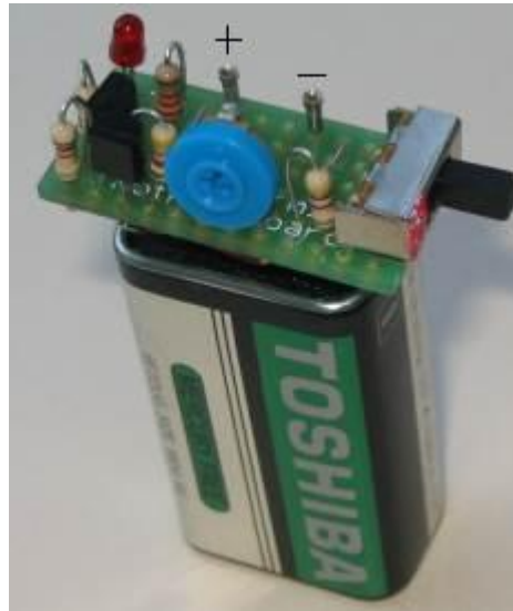
The regulator connected to a 9v battery
